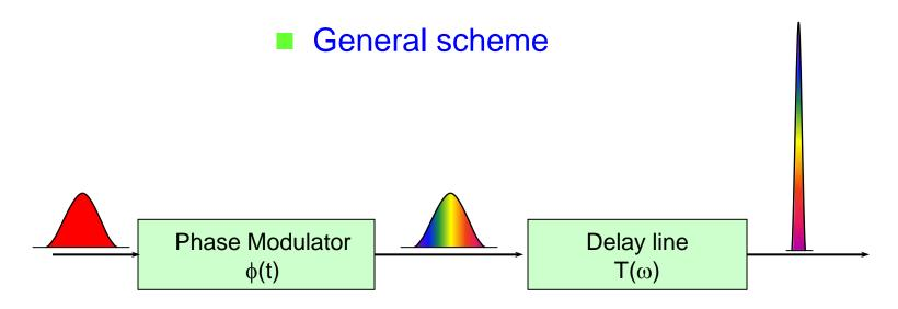
Phase Modulator ⇒ Self Phase Modulation (SPM)
