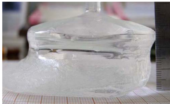
BBO crystal, grown from the fluoride flux, weighing 325 g
